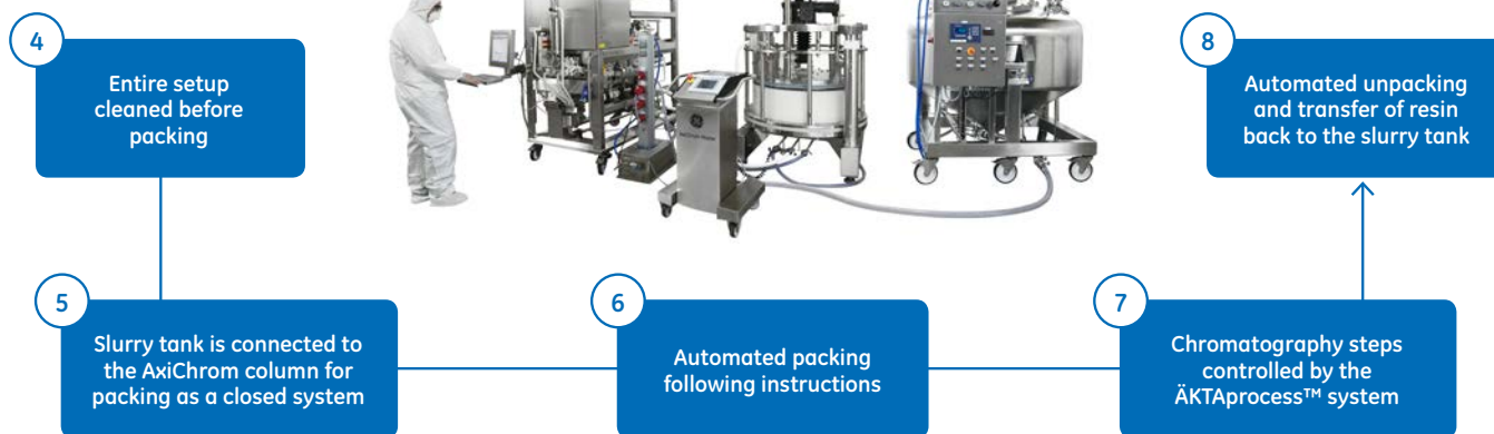
Fig 3. Contamination risks can be kept to a minimum by decreasing any manual handling of chromatography resin and buffers. This can be achieved by connecting the column, slurry tank and chromatography system in a closed system (blue boxes).
